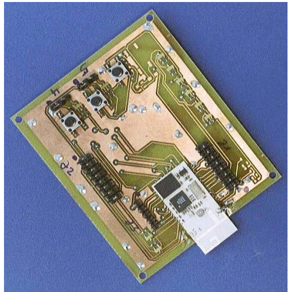
Figure 5: Evaluation board for LTCC BT-module
